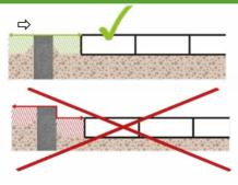
The ECORASTER® grid should be installed flush with the surface of the edge.
